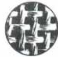
Multifilament weaves are made up of multiple stranded filaments twisted to form a single thread (*See Diagram*). The surface is rough, less uniform and the fabric is thicker. Photo emulsion adheres very nicely as do hand cut stencils. Thus multifilaments are suited for heavy ink deposits, offer excellent adherence for both knife cut stencils and photo process stencils. Also, multifilaments are usually readily available.
