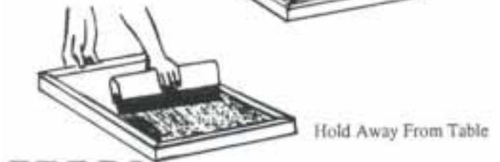
3. For a more durable screen, turn over and scrape coat the inside of the screen from bottom to top. Turn over and scrape coat inside of screen.
